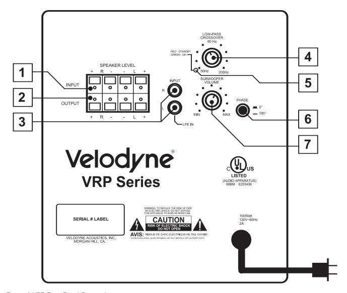
Figure 1.VRP Rear Panel Connections
